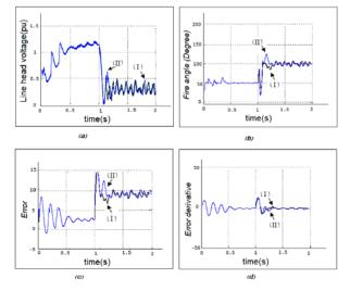
Figure 15. Performance comparison of Fuzzy-PD controller to both converters; a: line head voltage; b: fire angle; c: error; d: error derivative; (I: three phase fault on load; II: DC fault on transmission line)
