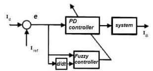
Figure 4. Rectifier control system (PD & FUZZY)
