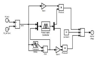
Figure 8. PD-Fuzzy rectifier controller
