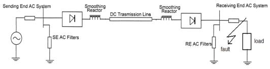
Figure 1. Single diagram of HVDC system with three- phase fault on load
