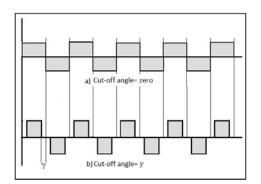
Figure 10. Cut-off angle for a phase
