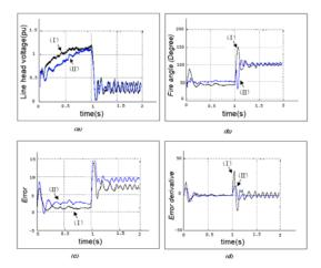
Figure 11. Comparison of performances of PD and Fuzzy-PD controllers; a: line head voltage; b: fire angle; c: error; d: error derivative; (I: PD controller on both converters; II: Fuzzy-PD controller on rectifier and PD controller on inverter)
