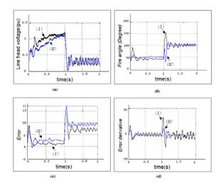
Figure 13. Comparison of performances of PD and Fuzzy-PD controllers; a: line head voltage; b: fire angle; c: error; d: error derivative; (I: PD controller on rectifier and Fuzzy-PD controller on inverter; II: Fuzzy-PD controller on rectifier and PD controller on inverter)
