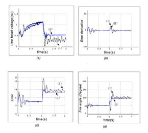
Figure 17. Performance comparison of Fuzzy-PD controller on both converters with three phase fault on load; a: line head voltage; b: error derivative; c: error; d: fire angle; (I: DC line length = 300 km; II: DC line length = 600 km)
