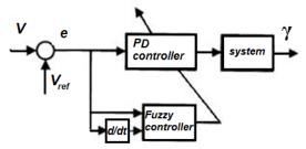
Figure 5. Inverter control system (PD & FUZZY)
