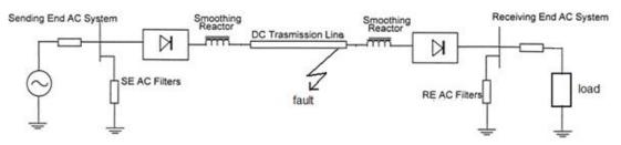
Figure 2. Single diagram of HVDC system with three-phas e fault on the DC line
