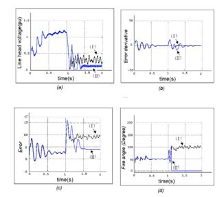
Figure 16. Performance comparison of Fuzzy-PD controller on both converters with three phase fault on load; a: line head voltage; b: error derivative; c: error; d: fire angle; (I: controller working continually; II: line power is disconnected when fault isn't removed)
