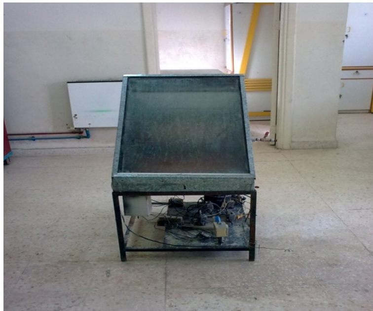
Figure 3 Experimental setup of a vacuumed solar still
