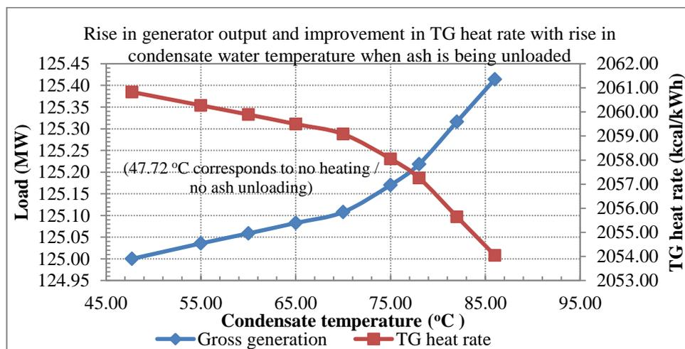
Figure 6. Gross turbine heat rate/ load vs condensate temperature
