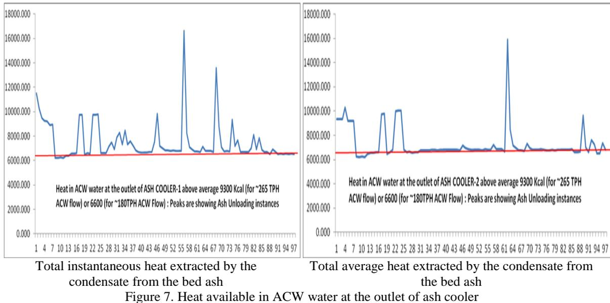
Heat available in ACW water at AC 1 & 2 is shown in Fig. 7(a) & (b). Total heat extracted is calculated by calculating area under the curve above a datum of 9300 kcal for ACW flow of 265 t/h and/or datum of 6600 kcal for ACW flow of 180t/h respectively at 36 °C ACW outlet temperatures. Probable risk factors and its remedial action are depicted in Table 4.
