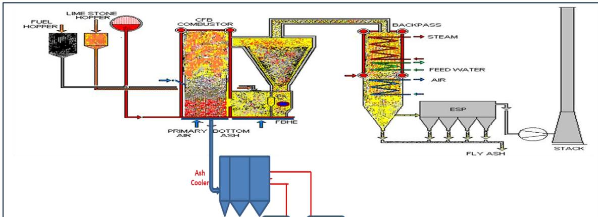
Figure 2. Basic lay out of the boiler.
