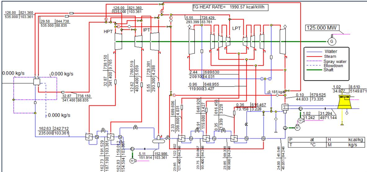
Figure 1. Heat and mass balance diagram based on manufacturer data.
