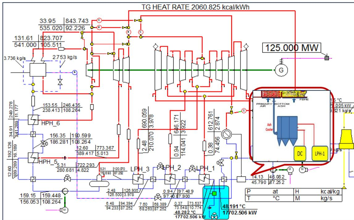
Figure 5. Proposed heat balance based on operating data
