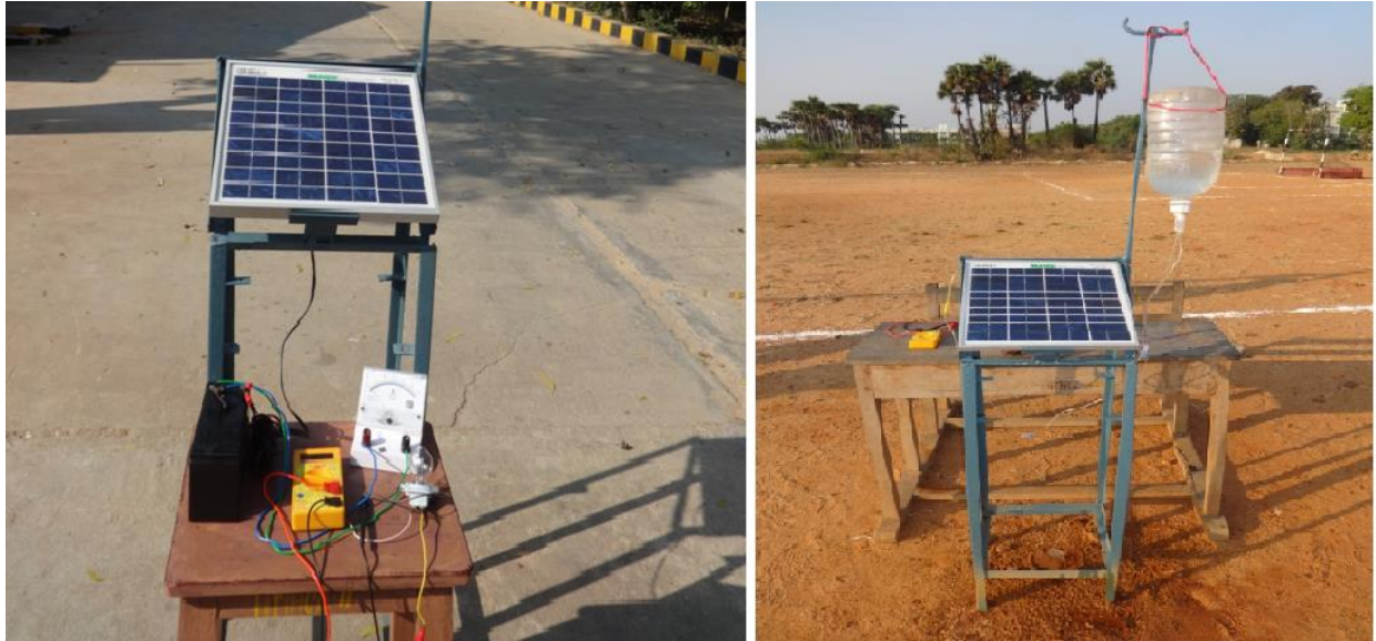
Figure 1. Photographic view of experimental setup with and without water cooling
