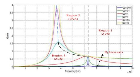
Figure 8. Frequency response of output voltage gain of the LLC resonant converter
