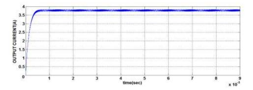
Figure 16. Output current of quasi resonant buck converter
