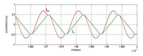
Figure 10. Output current at maximum power operating in region 2
