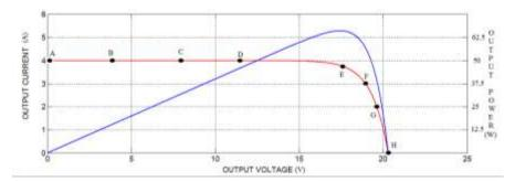
Figure 13. The V–I curve of the LLC resonant converter
