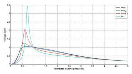
Figure 9. Frequency response of output voltage gain with different inductor ratios
