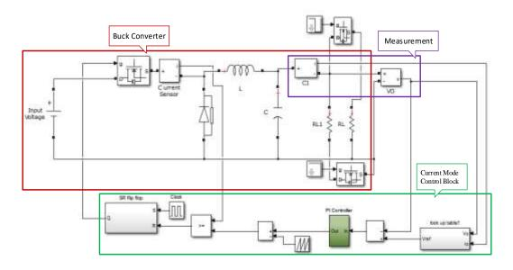
Figure 2. Simulink block diagram of current mode control of buck converter
