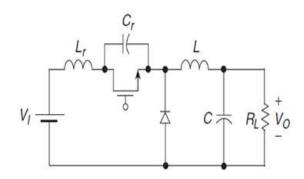
Figure 5. Circuit diagram of quasi resonant buck converter
