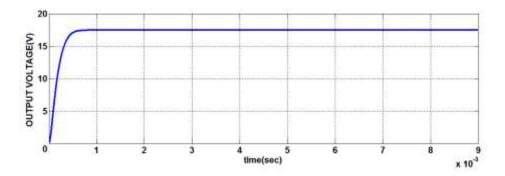
Figure 15. Output voltage of quasi resonant buck converter
