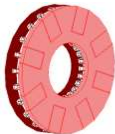
(a). Wound stator of generator
