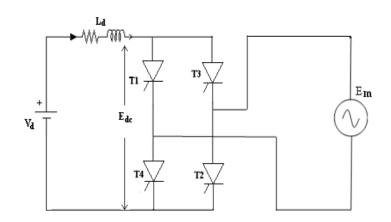
Figure 3. Circuit of the single-phase fully controlled bridge converter
