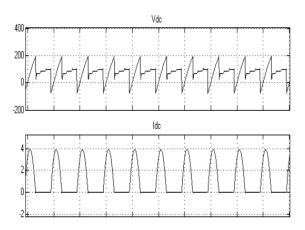
Figure 5. DC link voltage and DC link current
