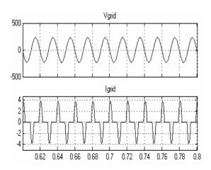
Figure 4. Grid voltage and grid current
