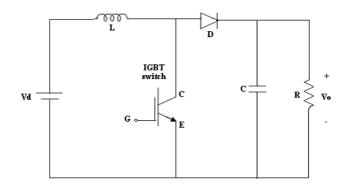
Figure 2. Circuit of the boost converter
