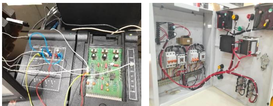
Figure 6. Simulation via Lucas Nuelle module and the wiring in panel
