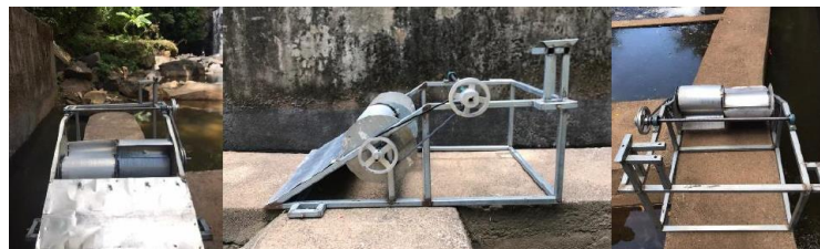
Figure 6. Construction result for series underwater Savonius rotor with horizontal axis
