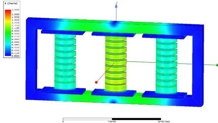
Figure 7. Distribution of magnetic flux density in the magnetic circuit
