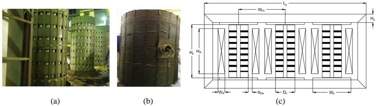
Figure 3. Geometry of a three phase SR (a) air gaps between core blocks, (b) winding structure, and (c) construction of a three phase SR
