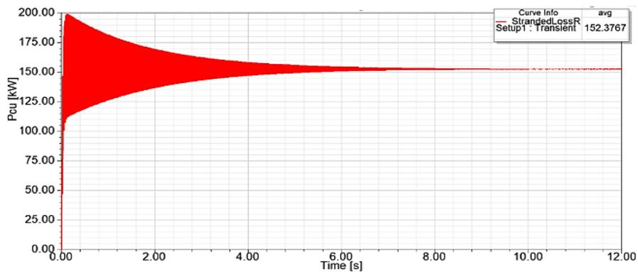
Figure 10. Copper loss in the winding of the SR
