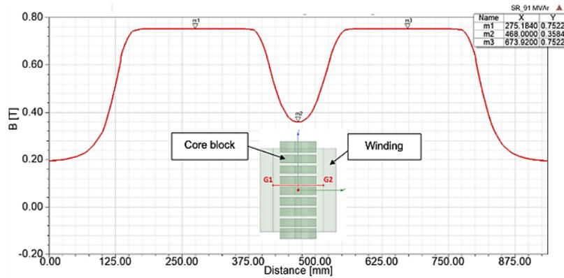
Figure 9. Magnetic flux density along the air gap (G1-G2) between core blocks
