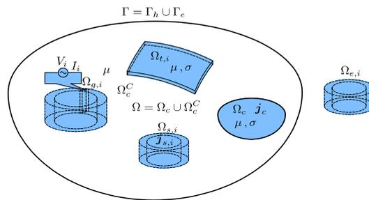
Figure 1. General magnetodynamic model [10]
