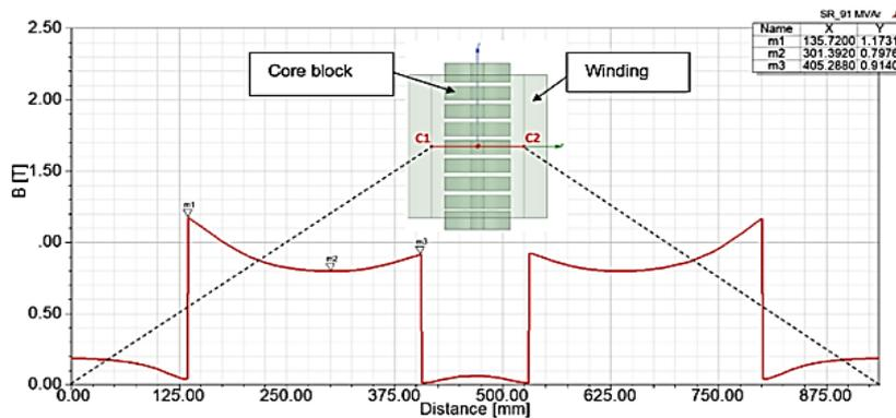
Figure 8. Distribution of magnetic flux density along the line of C1-C2 (core block)
