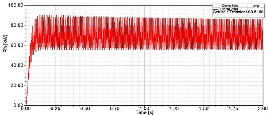
Figure 11. Iron loss in the magnetic circuit of the SR
