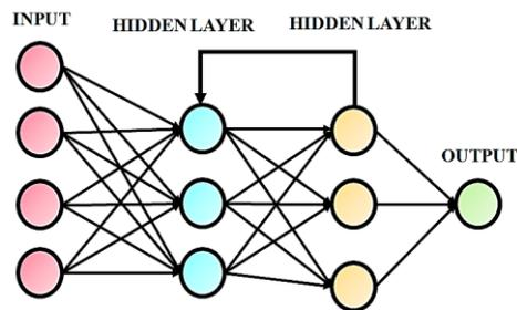
Figure 7. Structure of RNN based MPPT
