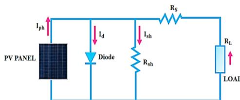
Figure 2. PV system model
