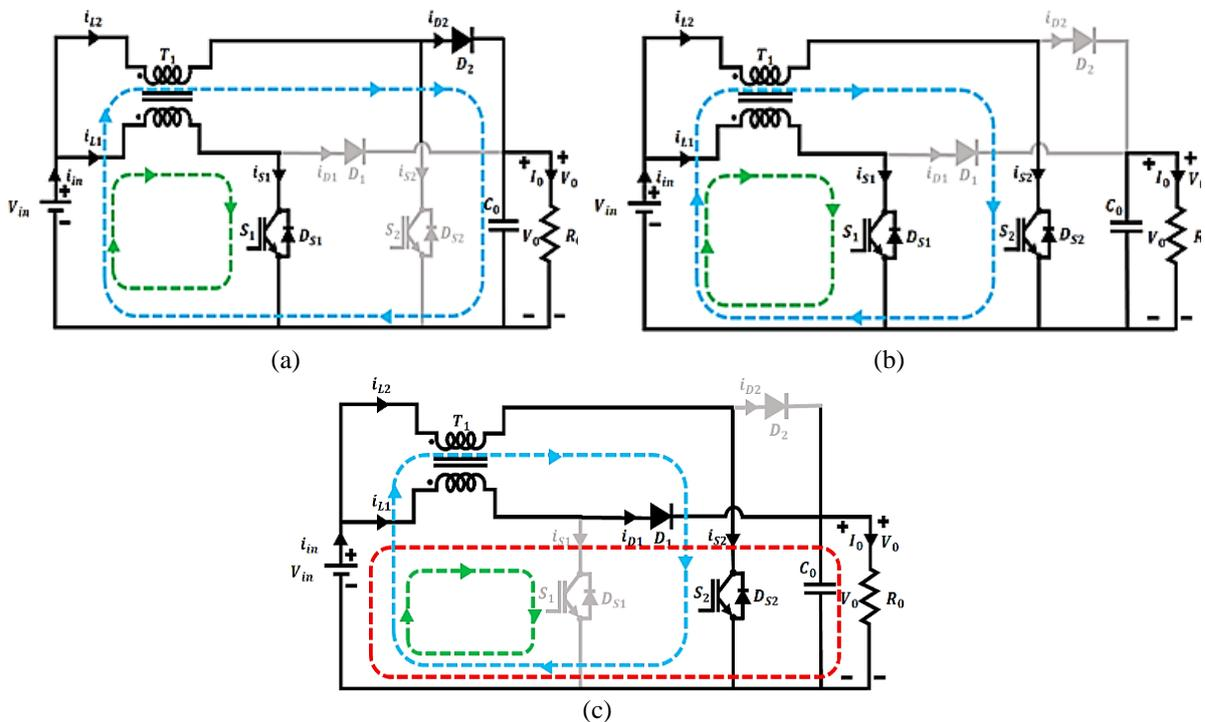
Figure 5. Modes of operation 5 (a) phase 1, (b) phase 2, and (c) phase 3
