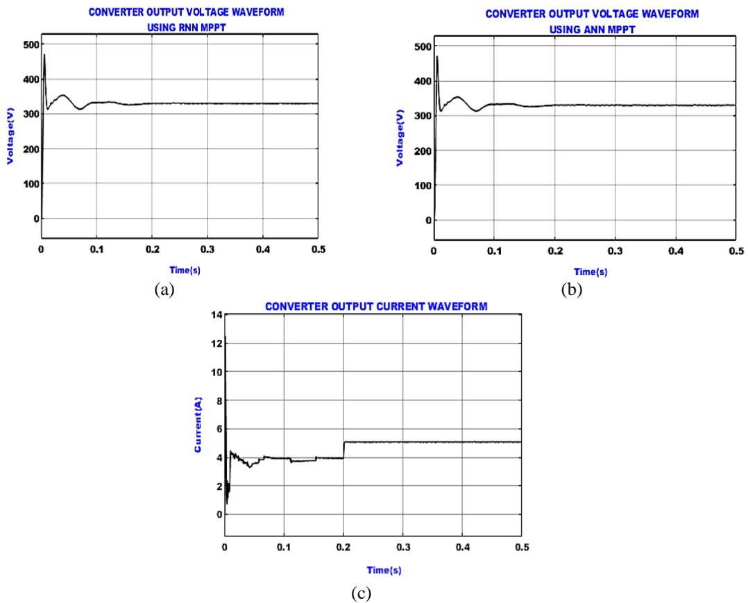
Figure 9. Waveforms representing the output voltage of converter using (a) ANN based MPPT, (b) RNN based MPPT, and (c) output current
