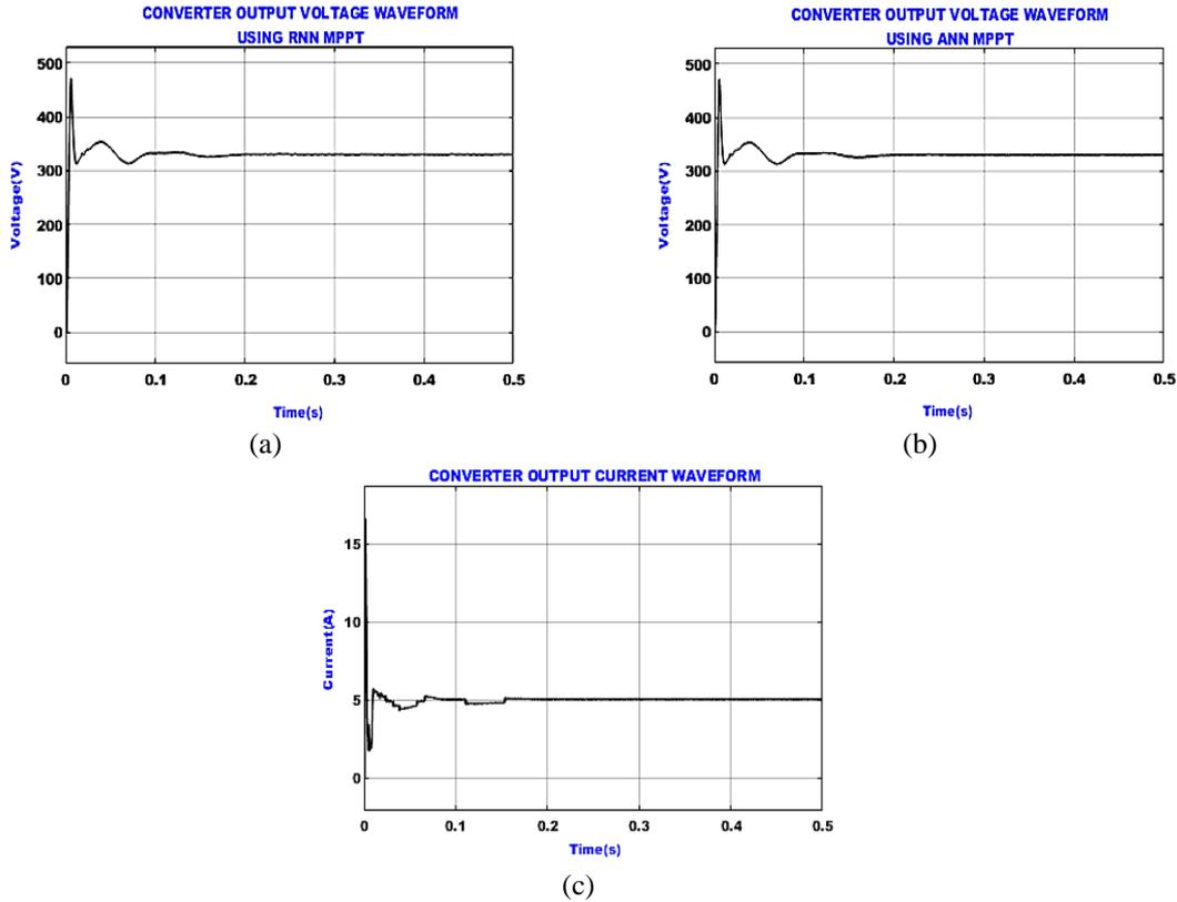
Figure 11. Waveforms demonstrating the output voltage of converter using (a) ANN based MPPT, (b) RNN based MPPT, and (c) output current
