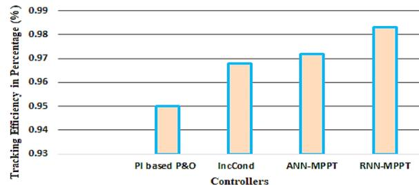
Figure 13. Comparison analysis of tracking efficiency
