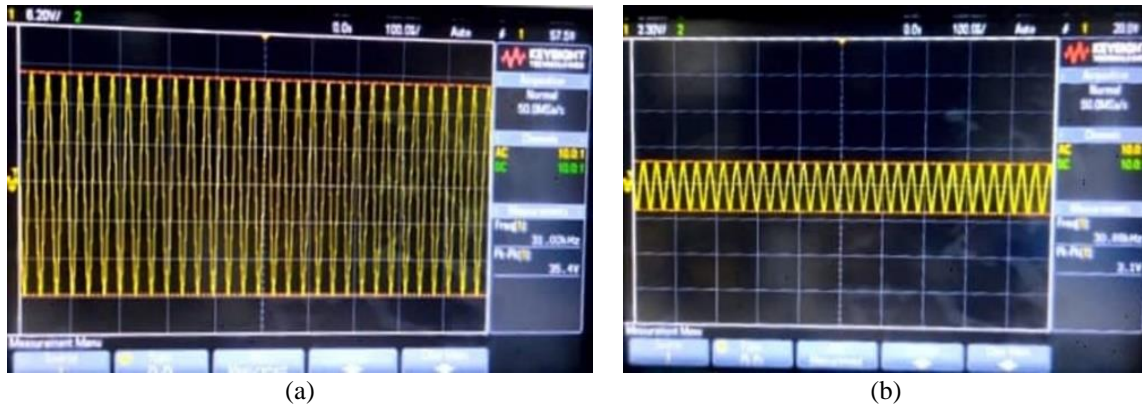
Figure 11. Voltage waveform in the receiver coil, when the distance between transmitter and receiver coil is (a) minimum and (b) maximum
