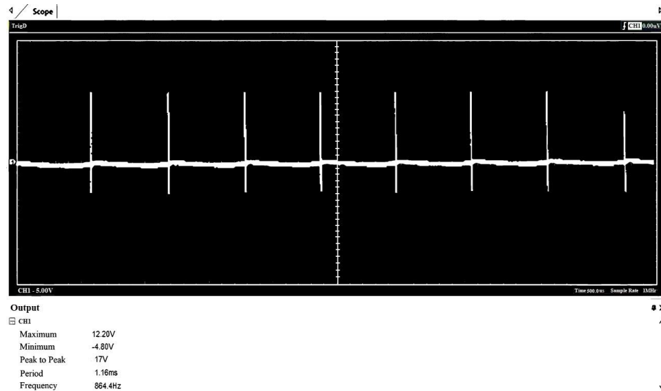
Figure 7. 5 Ah sulfated lead acid battery desulfation signal (500 us)
