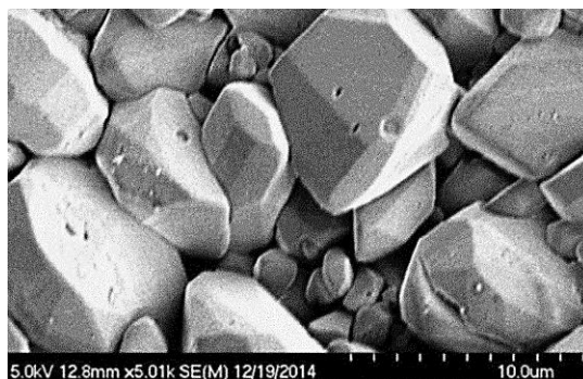
Figure 1. Micrograph of a sulfated electrode
