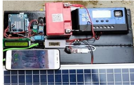
Figure 8. Solar cell based power-bank display tool
