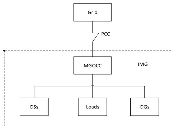
Figure 1. Islanded microgrid architecture
