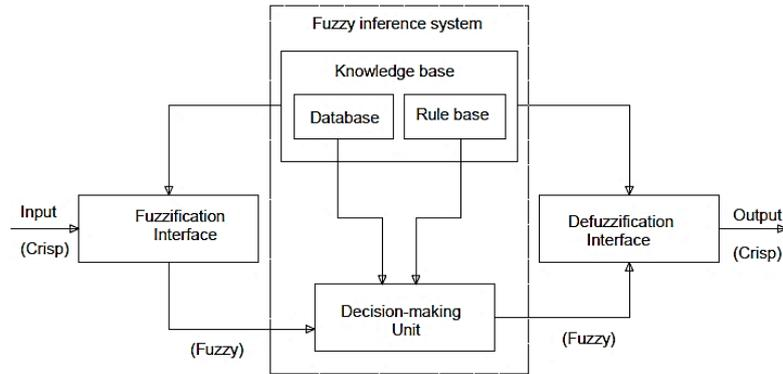
Figure 2. Fuzzy logic system architecture
