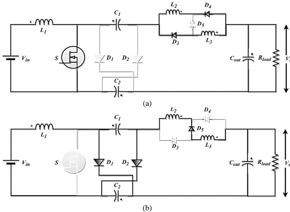
Figure 3. Modes of operation (a) mode 1 and (b) mode 2
