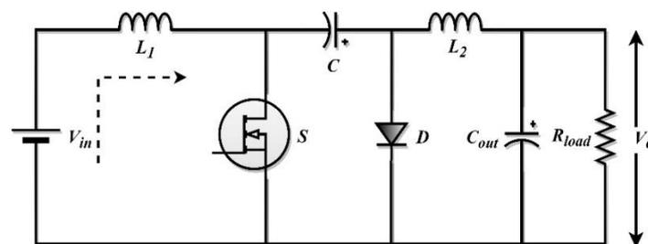
Figure 1. Schematic of the original Cuk converter
