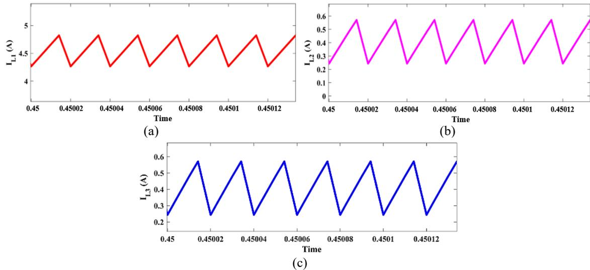
Figure 8. Current waveforms of the inductors (a)  $I_{L1}$ , (b)  $I_{L2}$ , and (c)  $I_{L3}$
