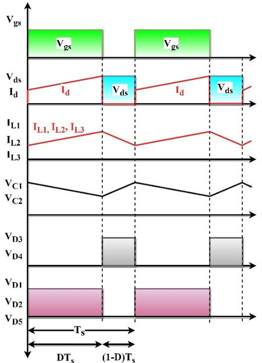
Figure 4. Theoretical waveforms of the proposed converter under CCM
