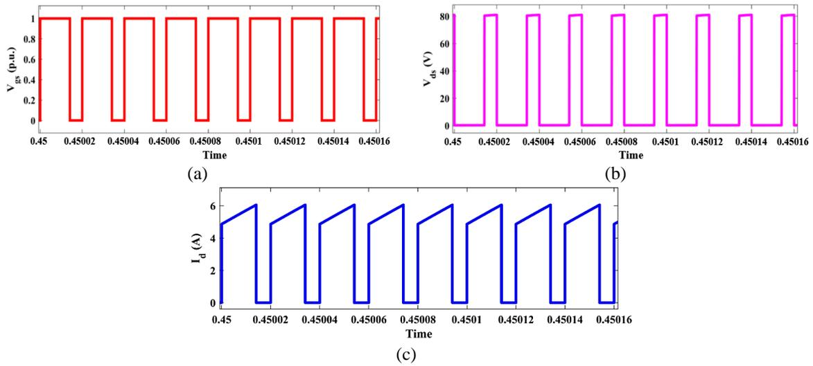
Figure 6. Current and voltage waveforms of the MOSFET (a) gating signal, (b) voltage stress, and (c) current stress
