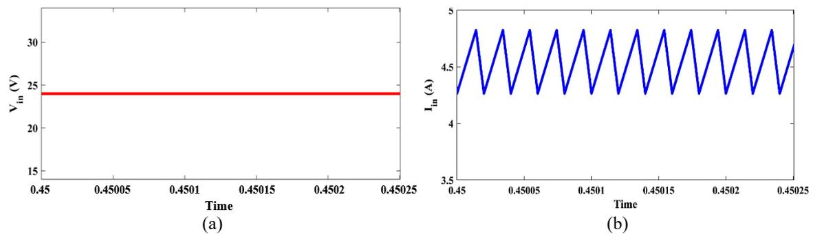
Figure 10. Source current and voltage waveforms (a)  $V_{in}$  and (b)  $I_{in}$
