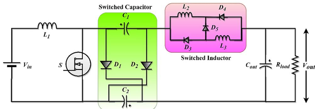
Figure 2. Schematic of the proposed MCKU converter
