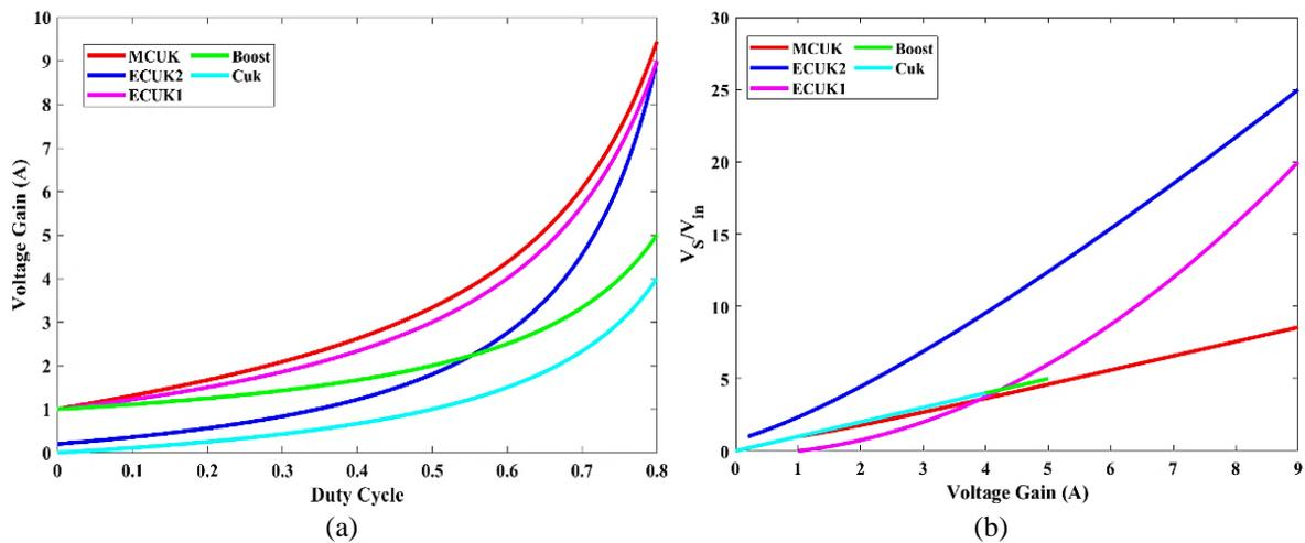
Figure 5. Performance comparison (a) output voltage gain and (b) voltage stress of the MOSFET
