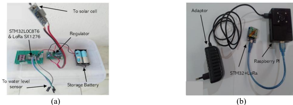
Figure 9. Realization of IoT devices: (a) sensor node and (b) gateway and server
