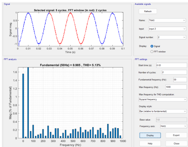
Figure 24. FFT voltage wave analysis after DVR placement at point 5
