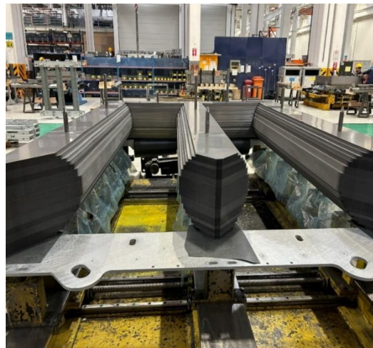
Figure 12. Core-making process in transformer manufacturing
