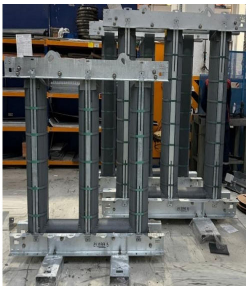
Figure 19. Comparison of transformer cores at 400 kVA and 1200 kVA
