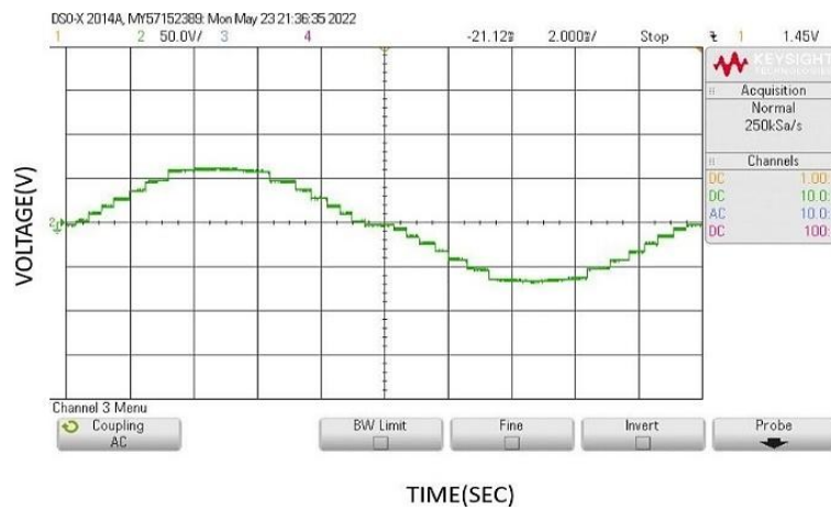
Figure 11. Output voltage - 15-level MLI – R load
