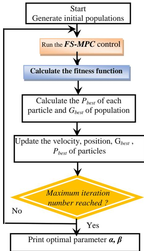
Figure 12. Flowchart of the PSO-  $\alpha\beta$  control
