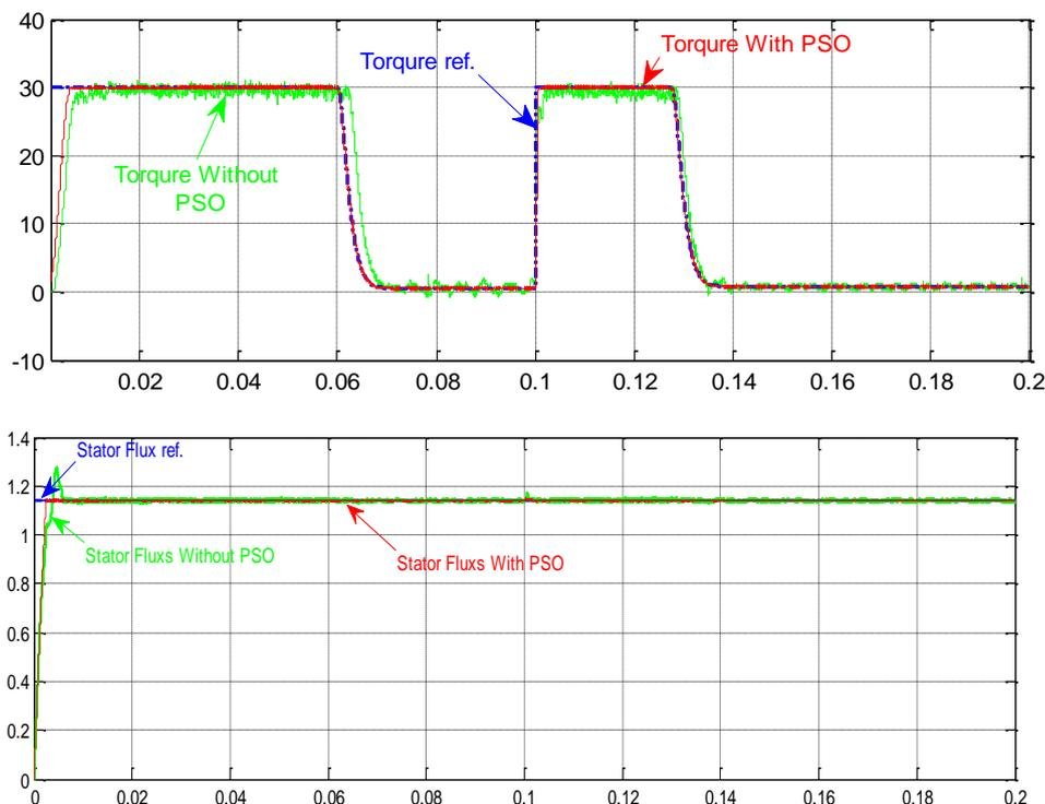
Figure 15 (a, b). Simulation results of torque and Stator flux with and without PSO
