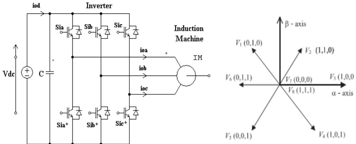
Figure 2. Two level source inverter with different voltage vectors
