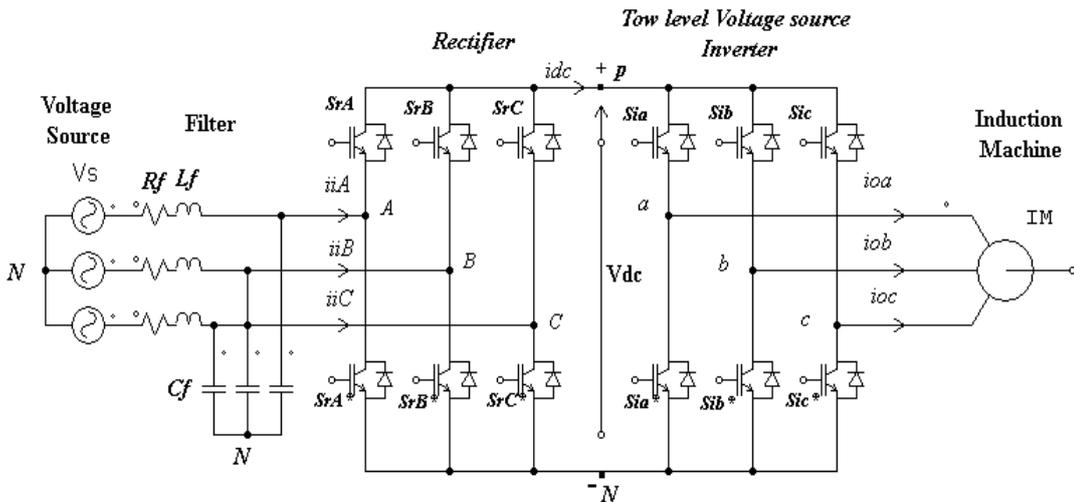
Figure 6. Indirect Matrix Converter (IMC) power topology.
