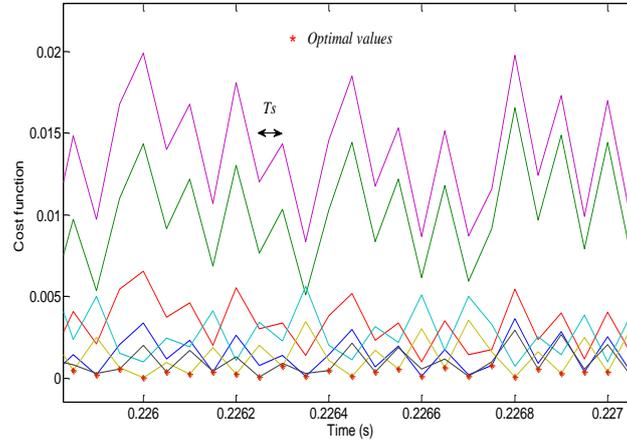
Figure 3. Selection of the optimal voltage vector for Cost function optimization in a two-level Voltage source inverter with FS-MPC control
