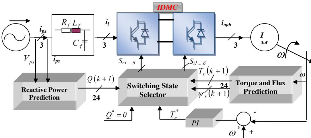
Figure 7. Predictive Indirect Power Control P-IPC control scheme without energy storage (Matrix Converter)
