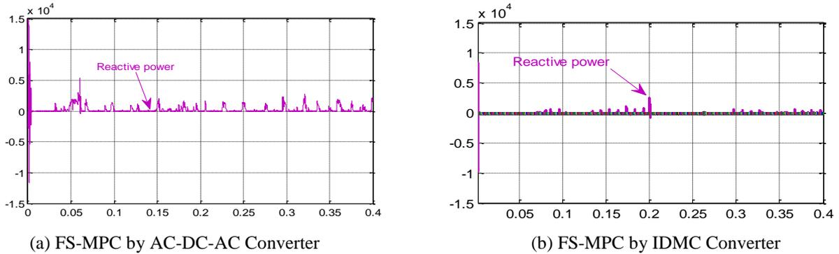
(a) FS-MPC by AC-DC-AC Converter (b) FS-MPC by IDMC Converter
