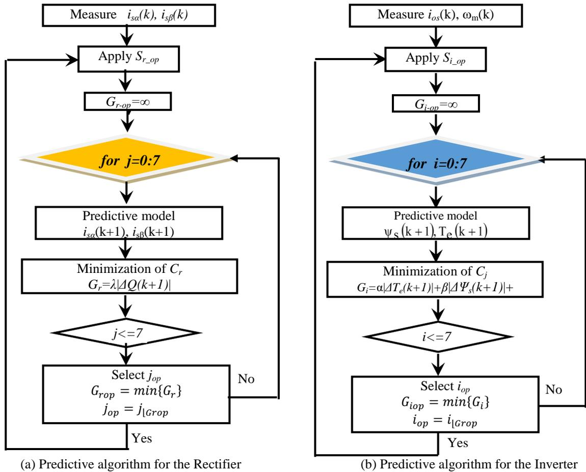
Figure 4. Flow chart of the predictive algorithm.
