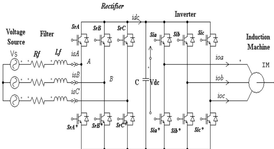
Figure 1. Indirect Converter (AC/DC/AC) power topology With energy storage
