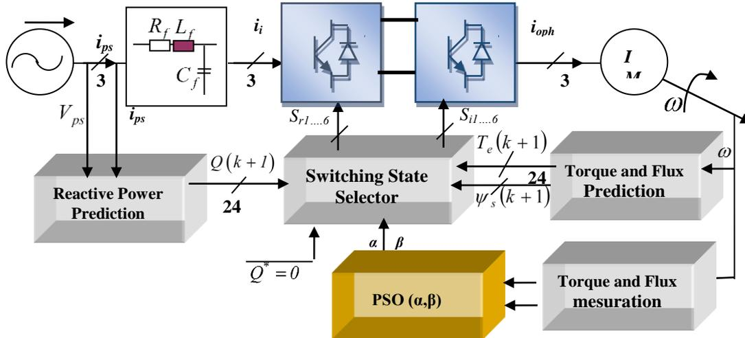
Figure 11. Scheme of predictive torque and flux control using PSO
