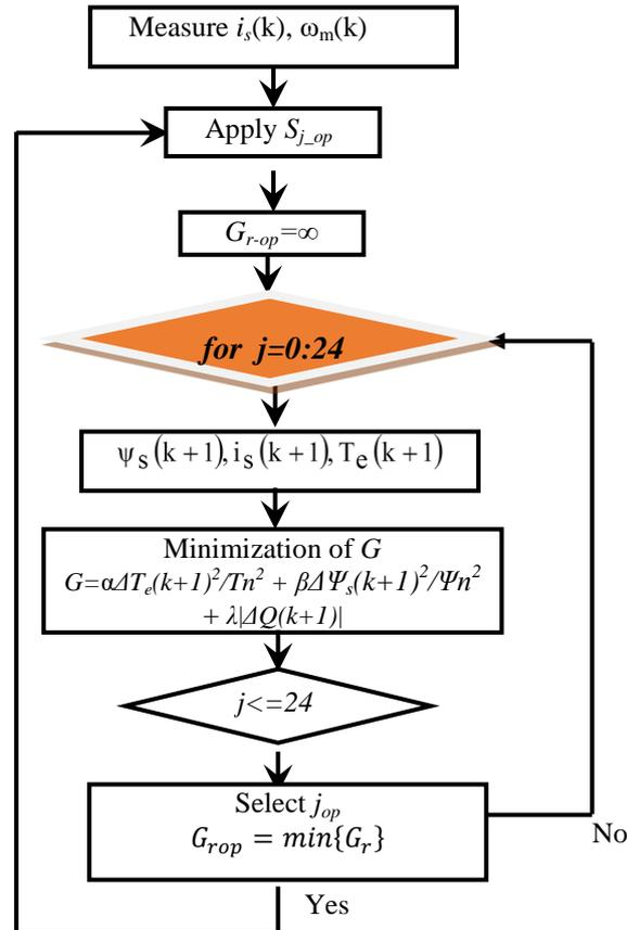
Figure 8. Predictive control algorithm with Indirect Matrix Converter
