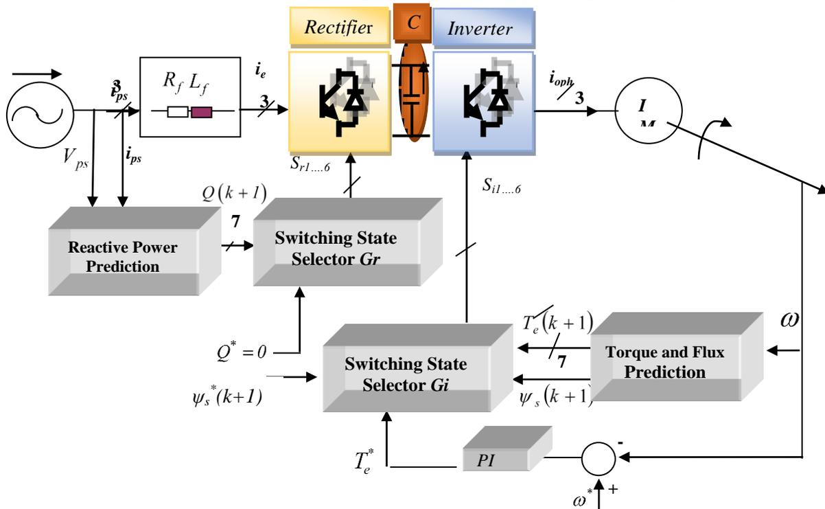
Figure 5. Predictive Indirect Power Control P-IPC control scheme with energy storage
