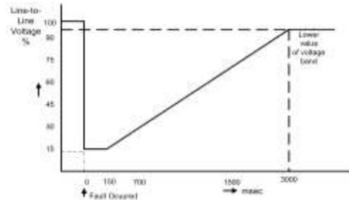
Figure 3. Typical low-voltage ride through requirement
