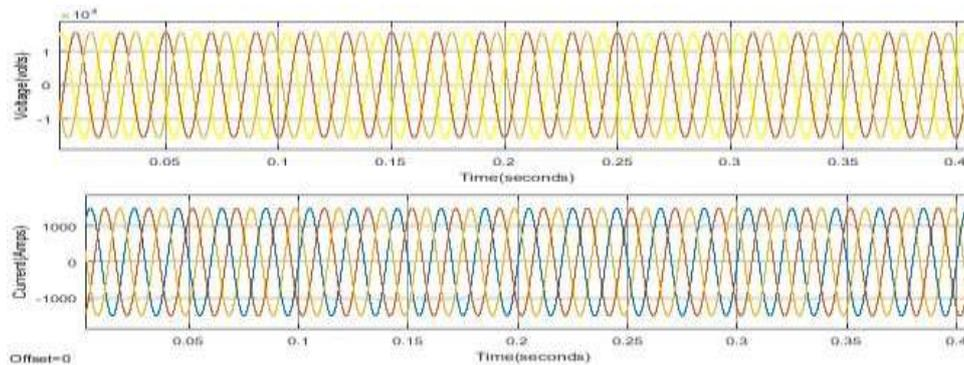
Figure 7. Local load voltage=11kV; current=1485.5A (peak to peak)
