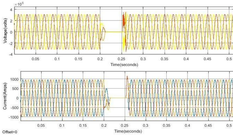
Figure 5. Grid side load voltage=220kV (rms), load phase current=927A (Peak to Peak)
