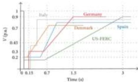
Figure 2. Low voltage ride through (LVRT) requirement in various grid codes in different countries
