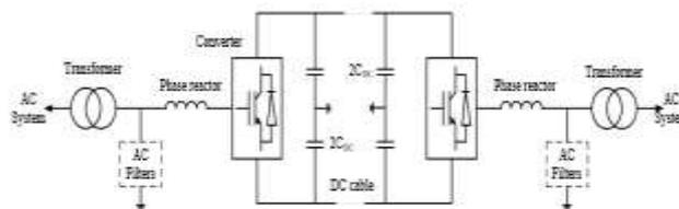
Figure 1. Typical VSC-HVDC system
